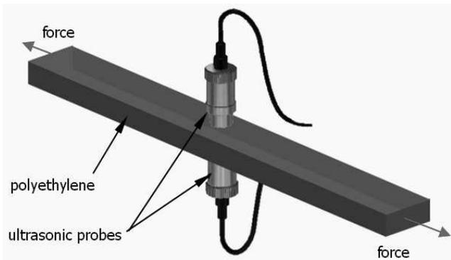
Fig. 1. Scheme of the ultrasonic testing
