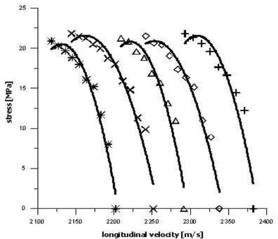
Fig. 3. Relationship between the stress and the ultrasonic wave in few specimens.
