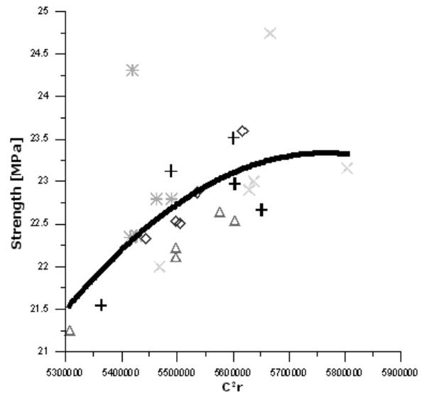
Fig. 2. Relationship between product of the ultrasonic wave velocity and density, and strength: + - speciment no boiling, ◇ - speciment after 48 hours of boiling; △ - speciment after 96 hours of boiling; × - speciment after 192 hours of boiling; \* - speciment after 288 hours of boiling
