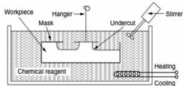
Fig. 1. Typical chemical machining set-up [6]
