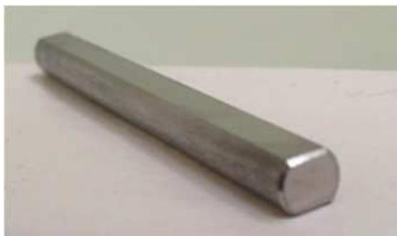
Fig. 1. Specimen of SAF 2205 stainless steel for surface treatments.
